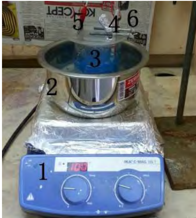
Fig. 2. The deposition setup, 1. Hotplate with magnetic stirrer, 2. Water bath, 3. Electrolyte, 4. Cathode, 5. Anode, 6. Thermocouple
