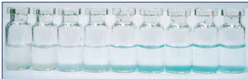
Figure 4.23 Naked-eyes of F- o BOH-AMP/Gd 3+ CNPs \subset copper(II) in HEPES (0.1M) pH 7.4 in the presence of different concentrations of cyanide anion. From left to right ( \times 10 \mu M): F- o BOH-AMP/Gd 3+ , 0, 2.0, 4.0, 7.0, 10.0, 20.0 30.0, and 40.0.
