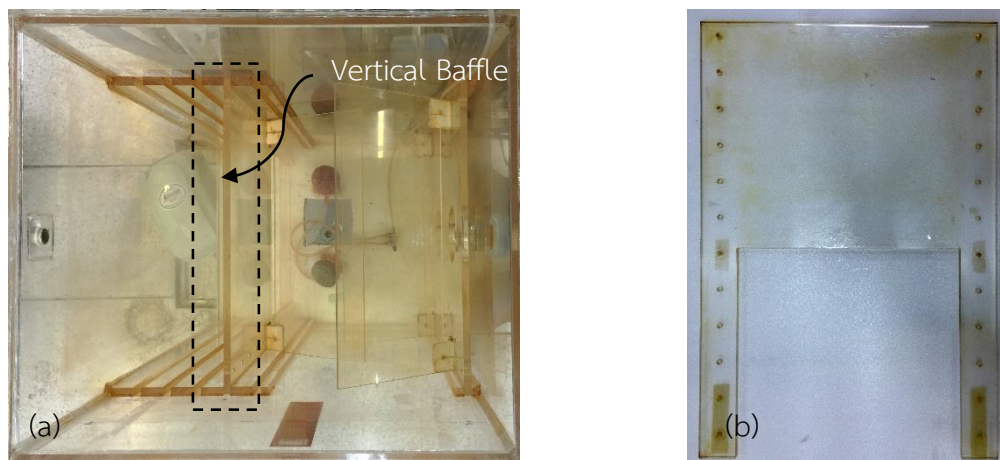
Figure 3.4. Fitted vertical baffle in the reactor top view (a) and vertical baffle flat (b) for changing from BCR to ALR
