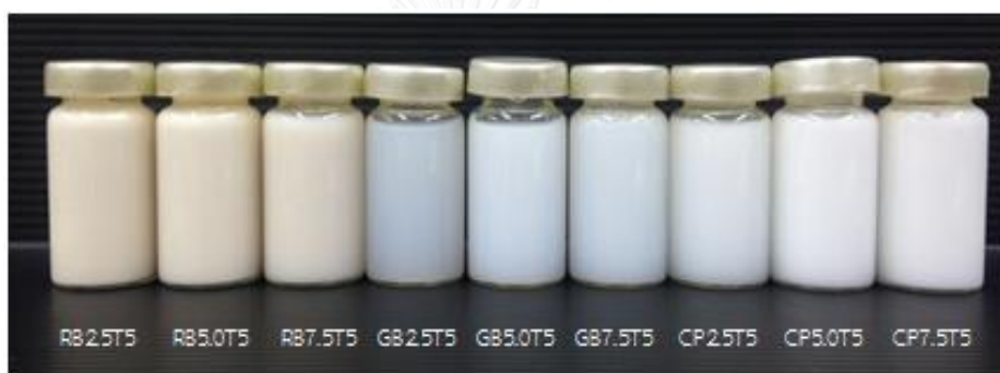
Figure 10. Appearances of freshly prepared blank-SLN: lipid 2.5, 5.0 and 7.5 (% w/w); tween 80 at 5 (% w/w) (RB = Rice bran wax, GB = Glyceryl behenate, CP = Cetyl palmitate, Tw = Tween 80)
