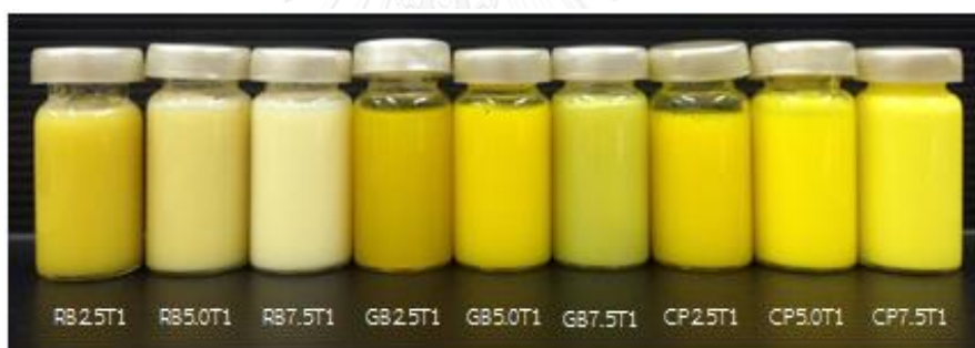
Figure 12. Appearances of freshly prepared C-SLN: lipid 2.5, 5.0 and 7.5 (% w/w); tween 80 at 1 (% w/w) (RB = Rice bran wax, GB = Glyceryl behenate, CP = Cetyl palmitate, Tw = Tween 80)
