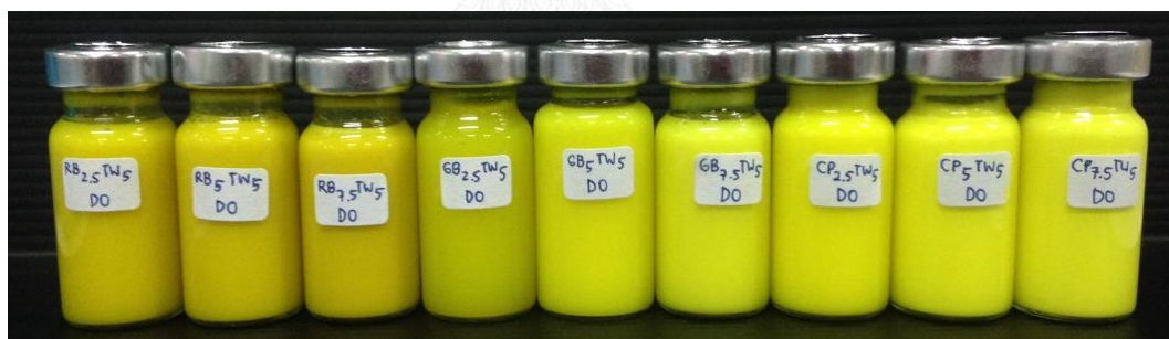
Figure 16. Appearances of freshly prepared BDMC-SLN: lipid 2.5, 5.0 and 7.5 (% w/w); tween 80 at 5 (% w/w) (RB = Rice bran wax, GB = Glyceryl behenate, CP = Cetyl palmitate, Tw = Tween 80)
