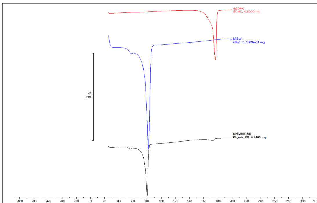
DSC thermograms of the Physical mixture of bulk lipid and drug (Rice bran wax: bisdemethoxycurcumin)
