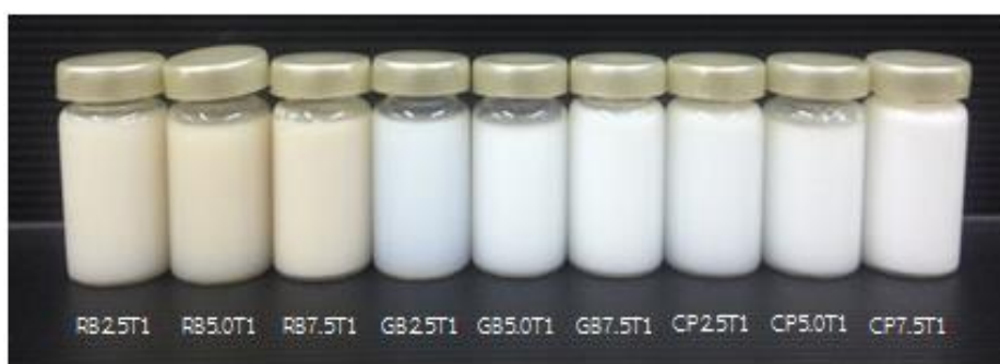
Figure 8. Appearances of freshly prepared blank-SLN: lipid 2.5, 5.0 and 7.5 (% w/w); tween 80 at 1 (% w/w) (RB = Rice bran wax, GB = Glyceryl behenate, CP = Cetyl palmitate, Tw = Tween 80)
