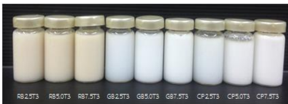
Figure 9. Appearances of freshly prepared blank-SLN: lipid 2.5, 5.0 and 7.5 (% w/w); tween 80 at 3 (% w/w) (RB = Rice bran wax, GB = Glyceryl behenate, CP = Cetyl palmitate, Tw = Tween 80)
