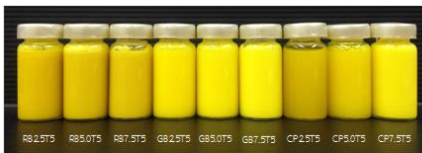
Figure 13. Appearances of freshly prepared C-SLN: lipid 2.5, 5.0 and 7.5 (% w/w); tween 80 at 5 (% w/w) (RB = Rice bran wax, GB = Glyceryl behenate, CP = Cetyl palmitate, Tw = Tween 80)
