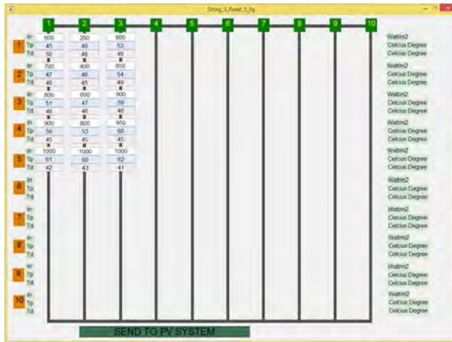
FIGURE B.2: The interface for user to set up the operating conditions of all panels. Each panel requires three input data: I_r, T_P, T_d . The button “SEND TO PV SYSTEM” updates the setting values to model in schematic for simulation.
