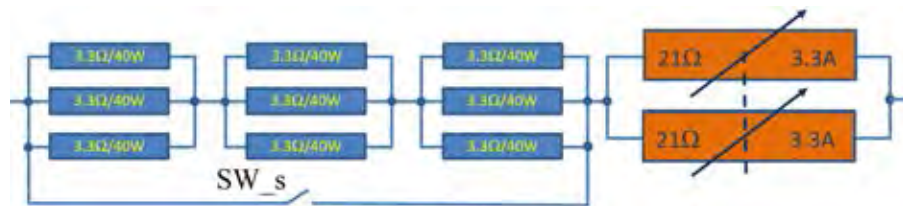
FIGURE 5.5: The variable load is used in scanning. The range of resistance is from 0 to 13.8\ \Omega . This range ensures that the MPP is tracked.
