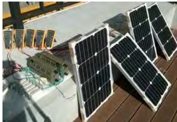
FIGURE 6.2: A string is composed of four mono panels STM6 – 40/36 of Solar Schutten manufacturer.
