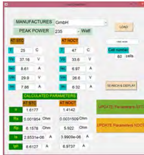
FIGURE B.9: Setting the parameters for solar cell follow model TS - 235PB - 60 of GmbH manufacturer.
