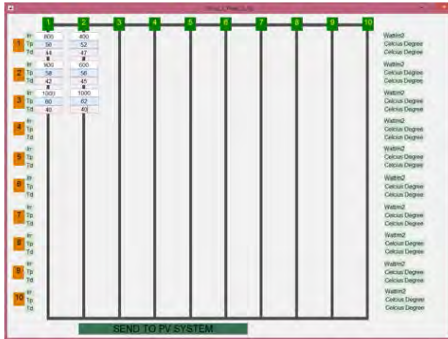
FIGURE B.10: Setting the operating conditions for all panels in 2x3 PV system.
