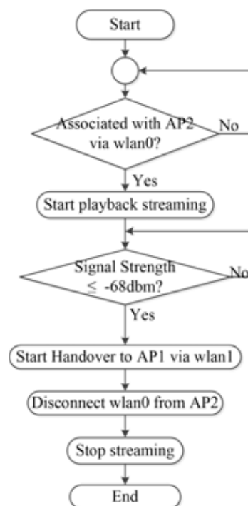
Figure 3.44: Event driven program of STA for client initiated handover processes using dual WLAN with 100% duplication.
