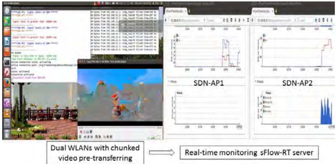
Figure 3.61: Video burst errors events at STA and sFlow-RT real-time monitoring graph for dual WLANs with chunked video pre-transferring.
