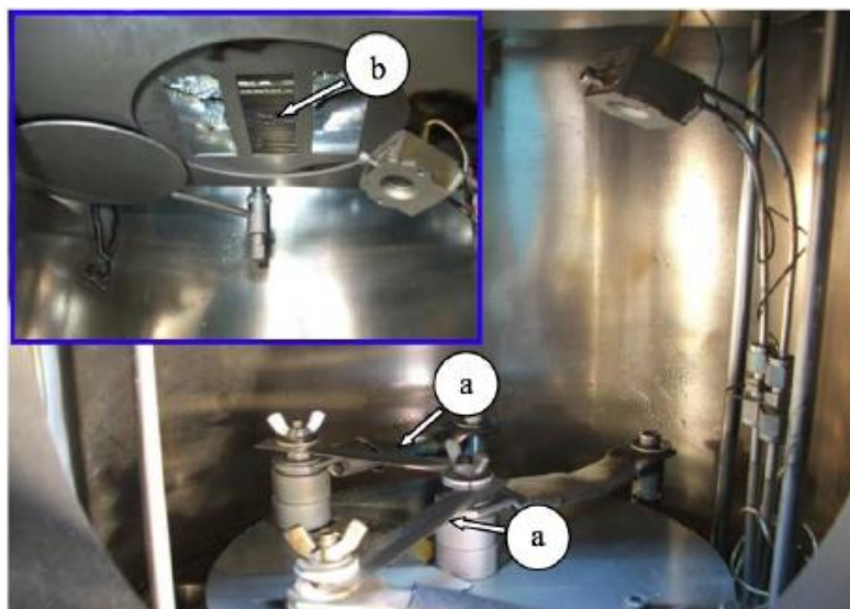
Figure 2.5 Instrument for cathode deposition. (a) tungsten boats and (b) 2 mm wide fingers of a shadow mask.
