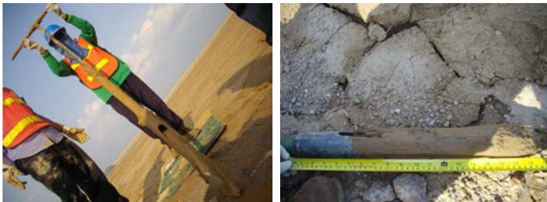
Figure 4.3 How to sample soil tailings samples from TSF area in each punch.
