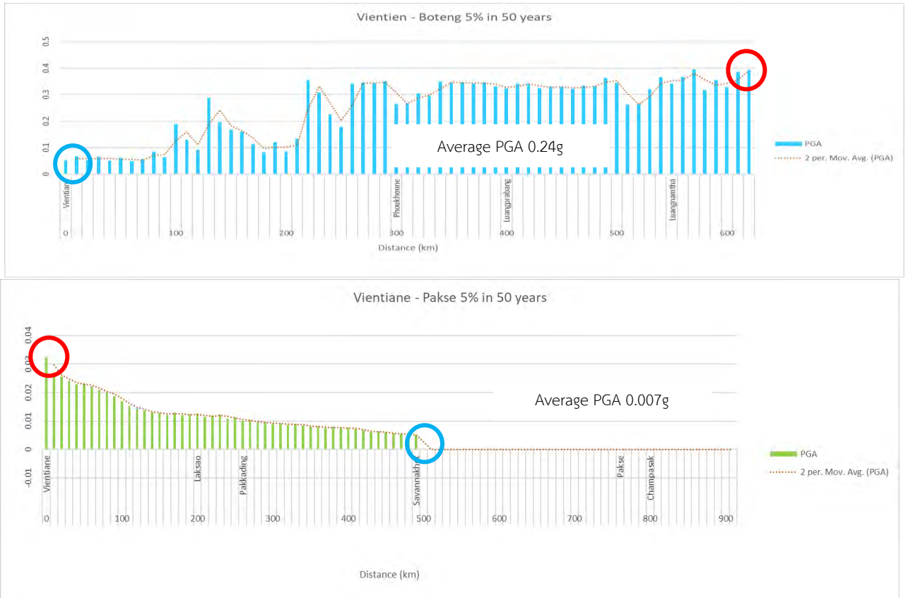
Figure 4.8. The charts show PGA values 5% POE 50 year along each line in Laos.
