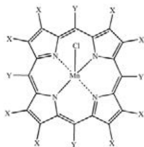
Figure 1.6 Structures of new ionophores manganese(III) porphyrin complexes. (12)
