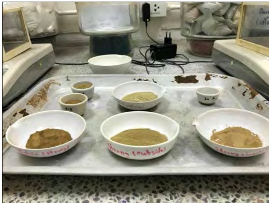
Figure 2.15 Powder samples prepare to steam in oven with 105° celcius to measure water content.
