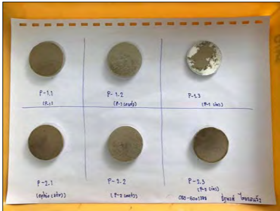
Figure 2.18 Sample packing for XRF analysis.
