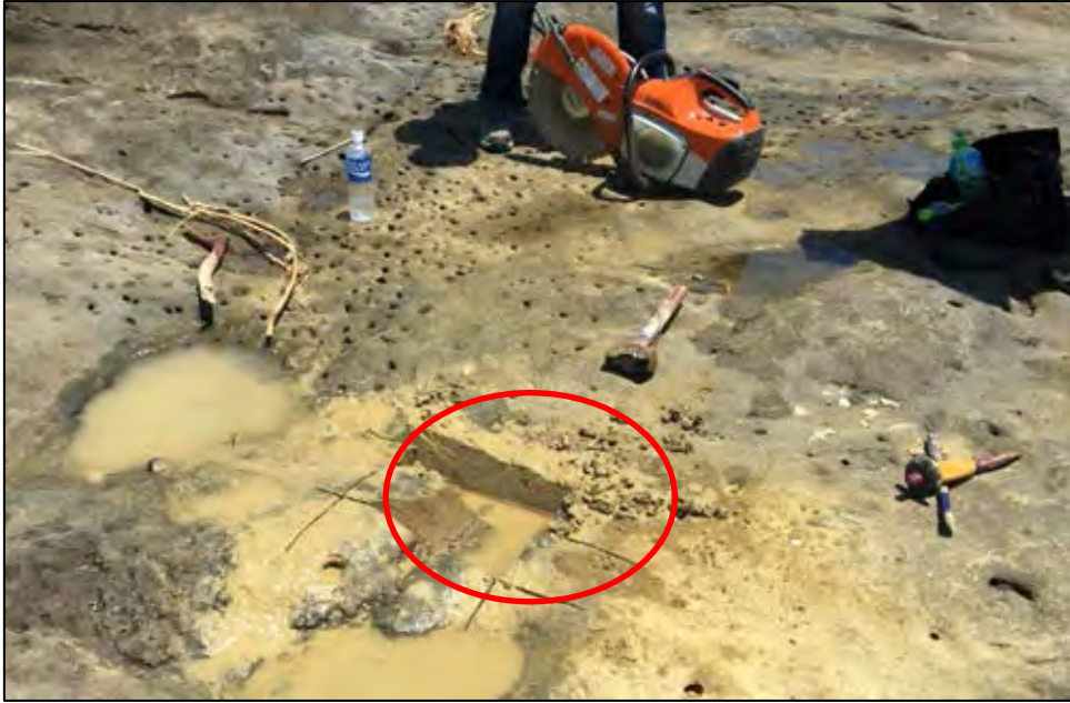
Figure 2.2 Equipment consists of automatic chainsaw (lubricated by water), chisel and hammer. Red circle shows the hole after sample collection.
