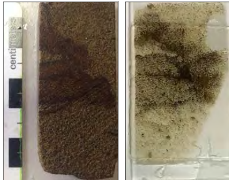
Figure 3.19 (Left) Ophiomorpha nodosa -dominated rock (from sample B) for preparing thin-section (Right) Thin-section of sample B
