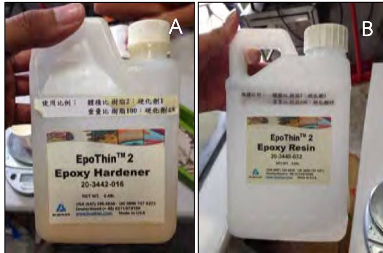
Figure 2.10 (A) Glue A is Epoxy hardener (B) Glue B is Epoxy resin.
