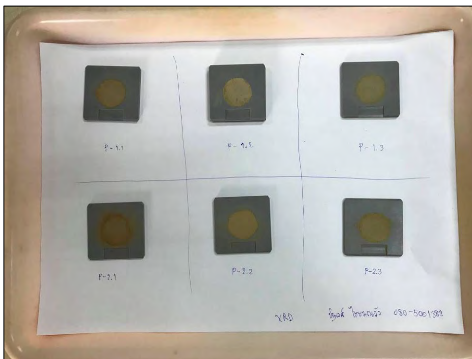
Figure 2.17 Sample packing for XRD analysis.
