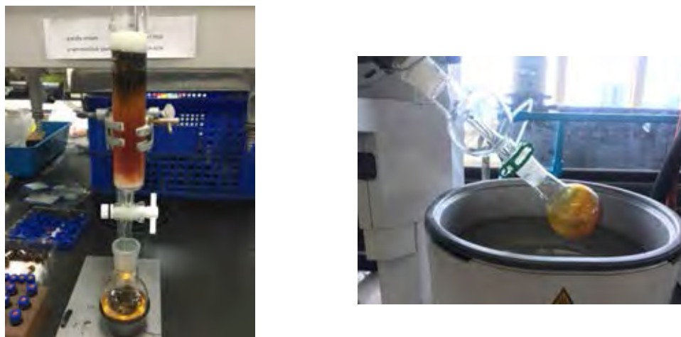
Figure 2.2 Photographs illustrating collection of fractions of green curry eluted from column chromatography (left) and evaporation of each fraction for solvent removal (right).
