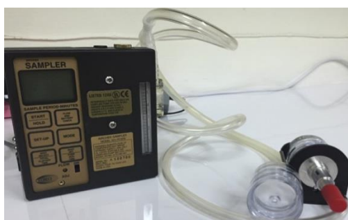
Figure 8 SKC personal sampling pump with cyclone and filter cassette
