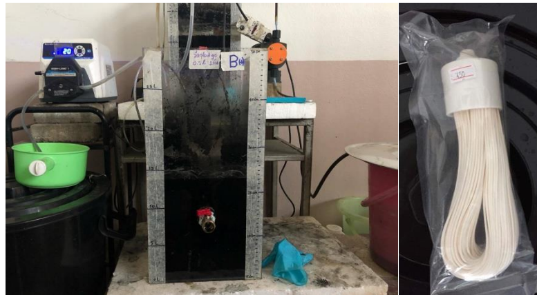
Figure 7. MBR tank and hollow fiber ultra-filtration membrane
