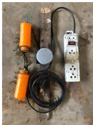
Figure 9. The float switch
