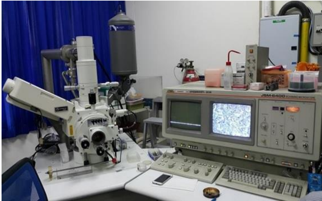
Fig 3.8 Scanning electron microscopy (SEM) model Jeol JSM-6400.
