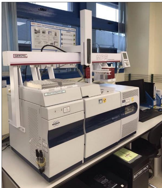
Fig 3.7 Gas-chromatography (GC) and Mass spectrometry (MS) model Bruker.
