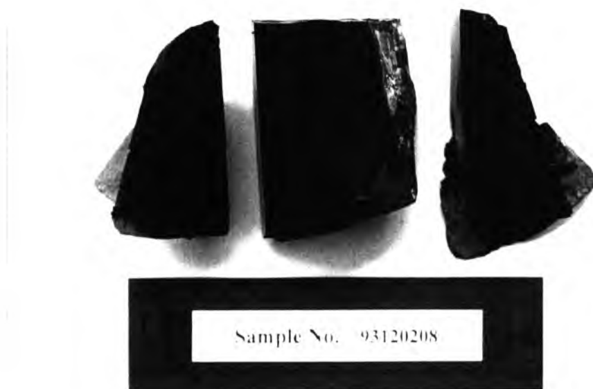
Figure 4.9 Light gray siltstone with blackish gray bands alternating of Carboniferous Hikoroichi Formation.
