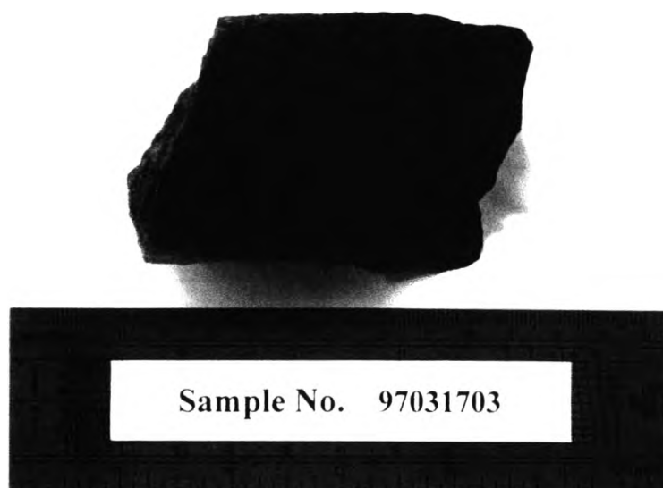
Figure 4.7 Well sorted fine-grained yellowish brown Triassic sandstone from Osawa Formation of Inai Group.
