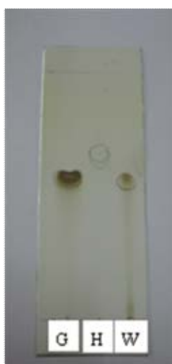
Figure 12. TLC chromatograms of standard gallic acid (G), the hexane extract (H) and the emblica extract (lyophilized powder) (W).
