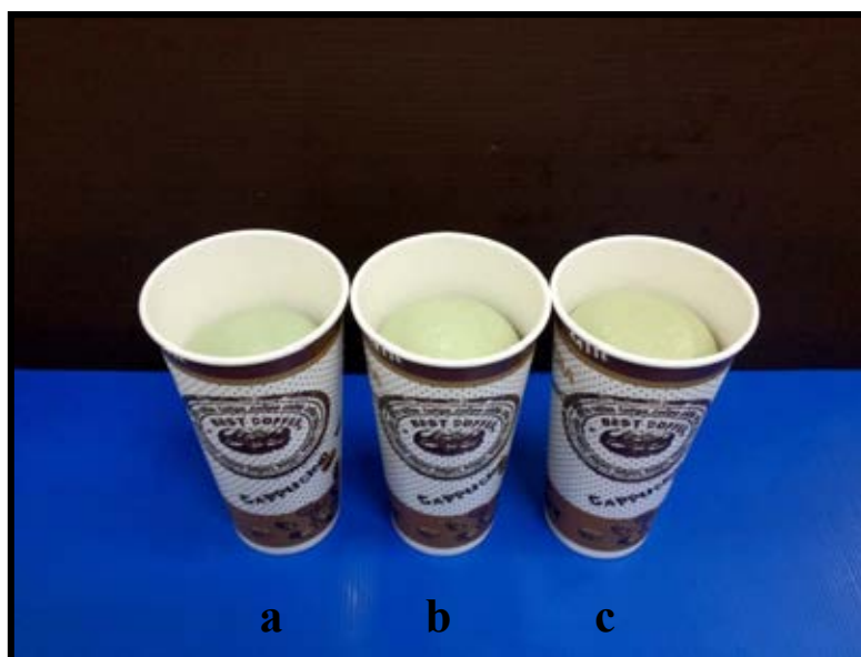
Figure 4.11 RPUR foams catalyzed by \text{Cu}(\text{NO}_3)_2 (tetraen) at different NCO indexes (a) 100; (b) 130 and (c) 150
