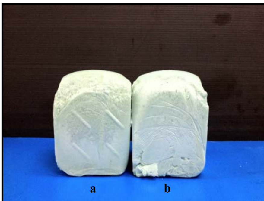
Figure 4.12 RPUR foams catalyzed by (a) \text{Cu}(\text{NO}_3)_2(\text{pentaen}) and (b) \text{Cu}(\text{NO}_3)_2(\text{tetraen}) prepared in a plastic mold
