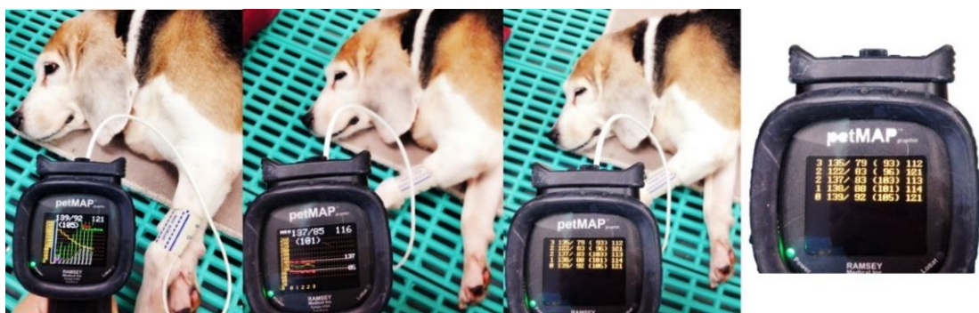
Figure 3-4 The instrumentation for the indirect blood pressure method, an oscillometric device (petMAP™, CardioCommand, Inc., Florida, USA) in experimental dog.
