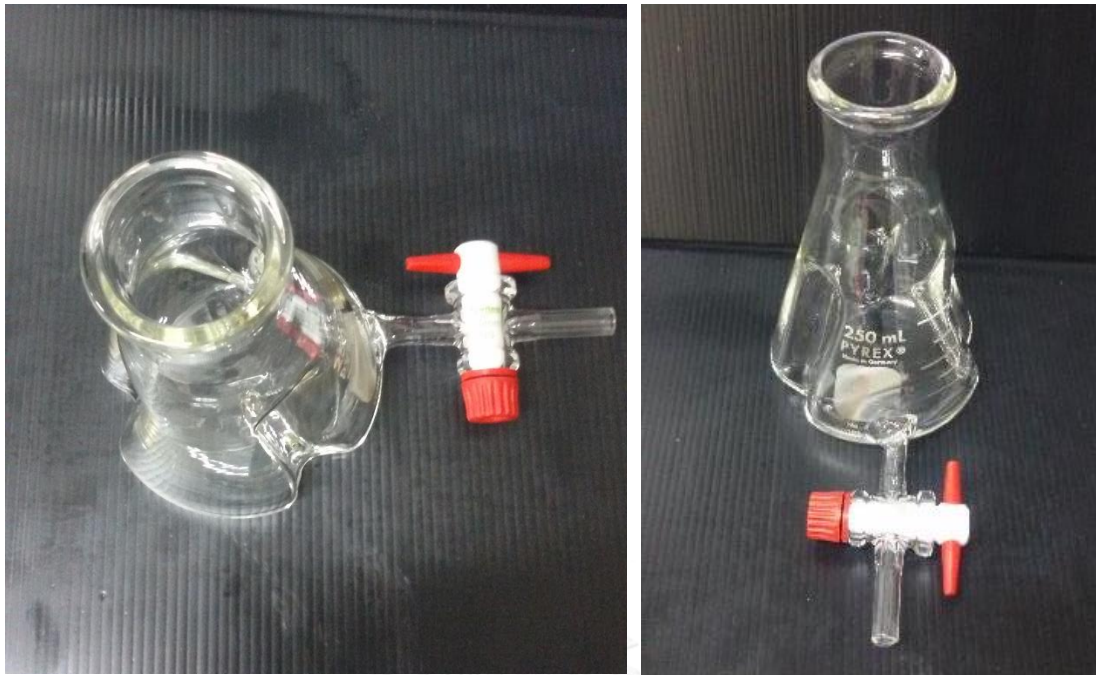
Figure 4.1 Photograph of the baffle flask for dispersant efficiency modified from Venosa et al. (2002) which had a stopcock at the bottom for taking the sample out.
