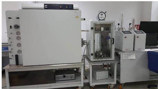
Figure 22. CFS-700 coreflooding system used in dynamic investigation of fluorescein solution with shaly-sandstone.
