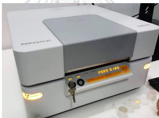
Figure 20. X-ray fluorescence (XRF) analyzer used in characterization of elemental composition of shaly-sandstone samples.
