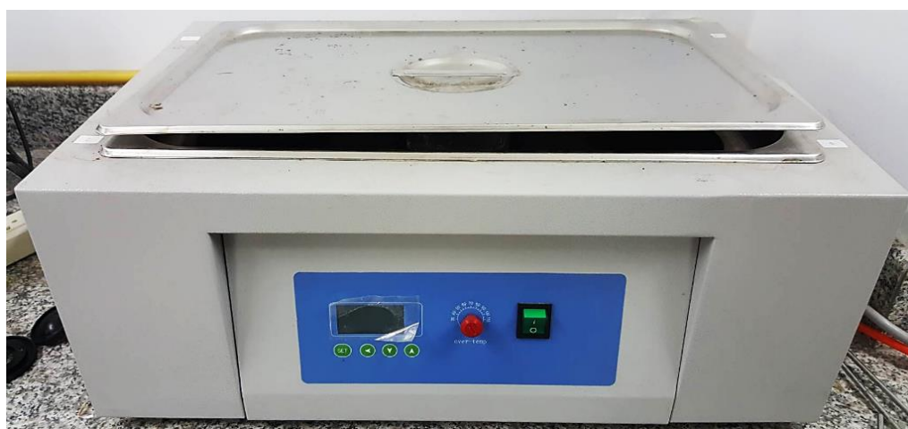
Figure 18. BWS-20 water bath used in determination of thermal stability of fluorescein solution.
