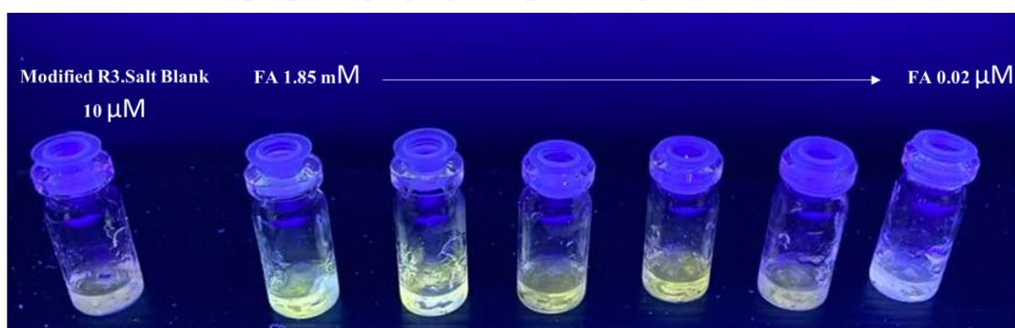
Figure 3.19 Fluorescence image of modified sol gel with 10 \mu\text{M} of R3.HCl upon adding formaldehyde 2 mM to 0.02 \mu\text{M} .
