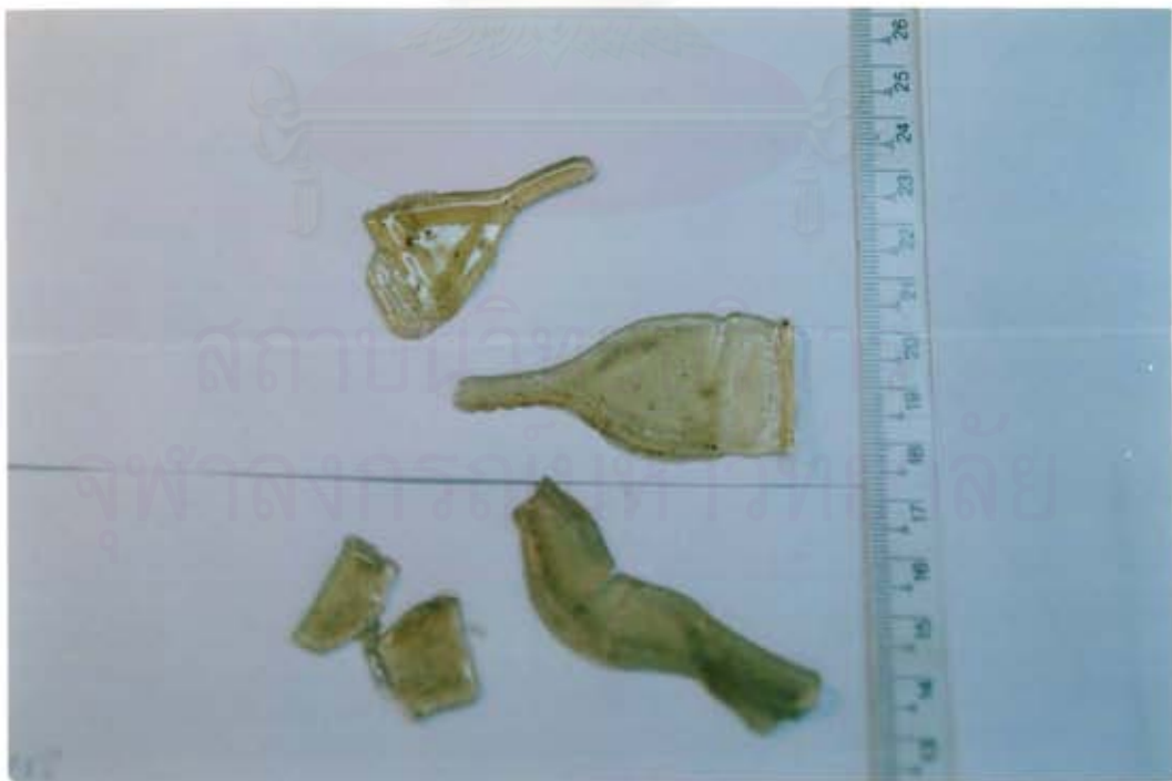
Figure 5.22 The appearance of I100 observed after 8 weeks of weathering test.
