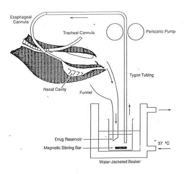
Figure 5 Schematic diagram of the in situ perfusion of the rat nasal cavity
