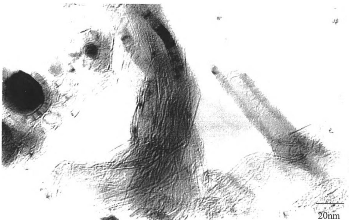
Figure 4.16 TEM image showing a mixture of SWNTs and MWNTs produced by methane decomposition on Co-Mo/MgO (1:1 mole ratio) catalyst at 900 °C
