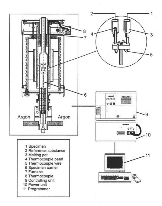
Fig.A1-1 Differential-Thermal Analysis (DTA) equipment.
