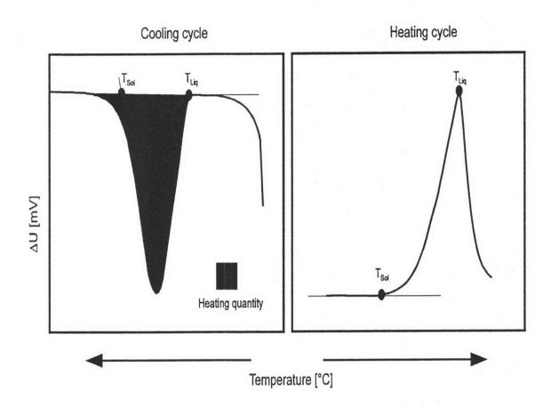
Fig.A1-2 Schematic diagram of a simple heating and cooling curve of DTA.
