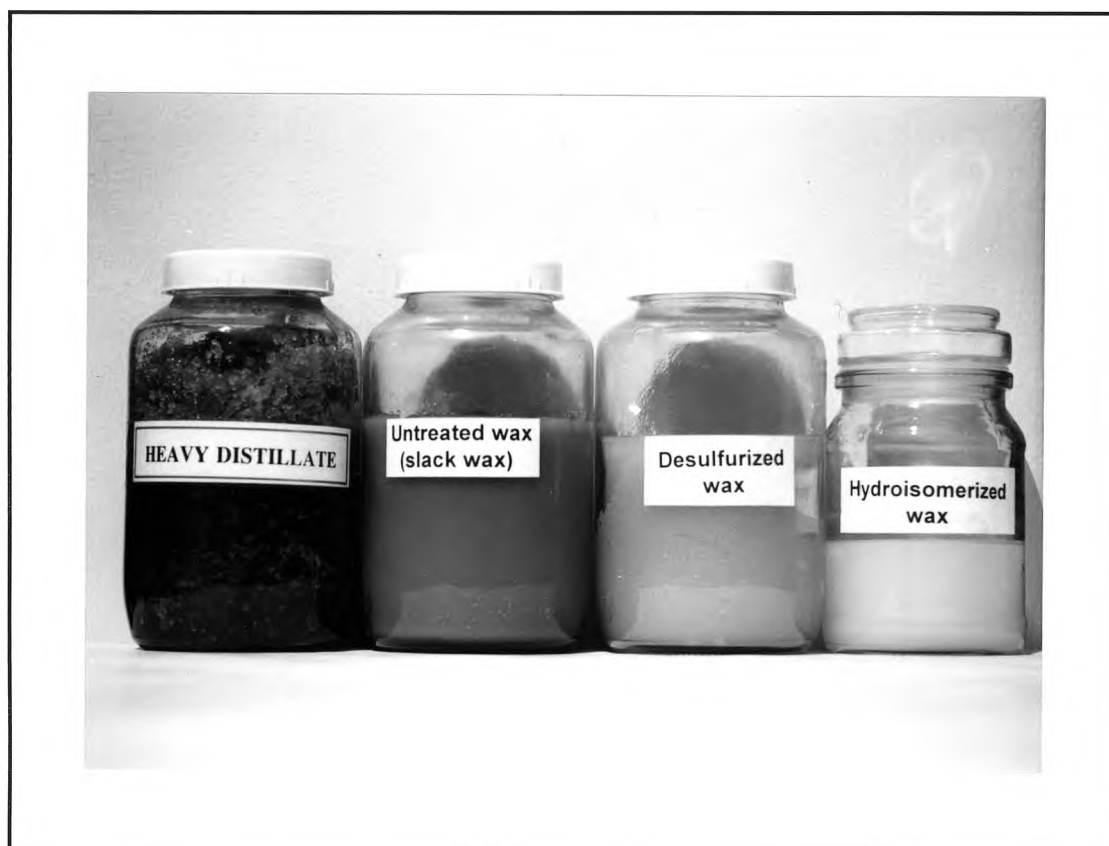
Figure 4.25 Fang heavy distillate, untreated wax (slack wax), desulfurized wax, and hydroisomerized wax
