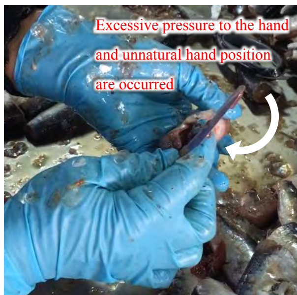
Figure 11 Excessive pressure and unnatural hand position occur when holding the spoon
