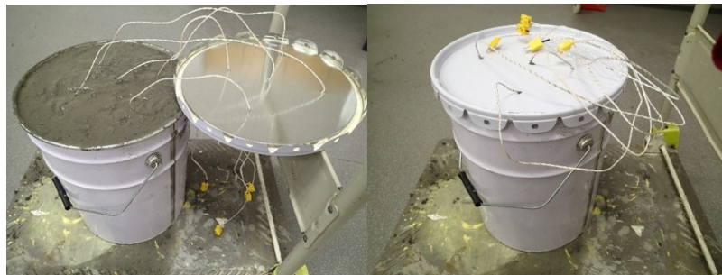
Figure 6. 20L Concrete sample for testing (before (left) and after (right) covering)
