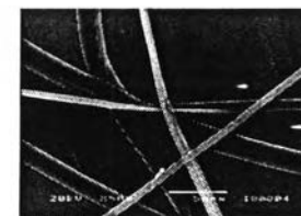
Figure 4.22 SEM images of as-spun fibers obtained from PS solutions at 10%, 20%, and 30% (w/v) in a mixed solvent of DMF and MEK in various volumetric ratios a) 100/0; b) 75/25; c) 50/50; d) 25/75; and e) 0/100. Applied electrical field was 20 kV/10 cm and the scale bar shown is for 50 \mu\text{m} .
