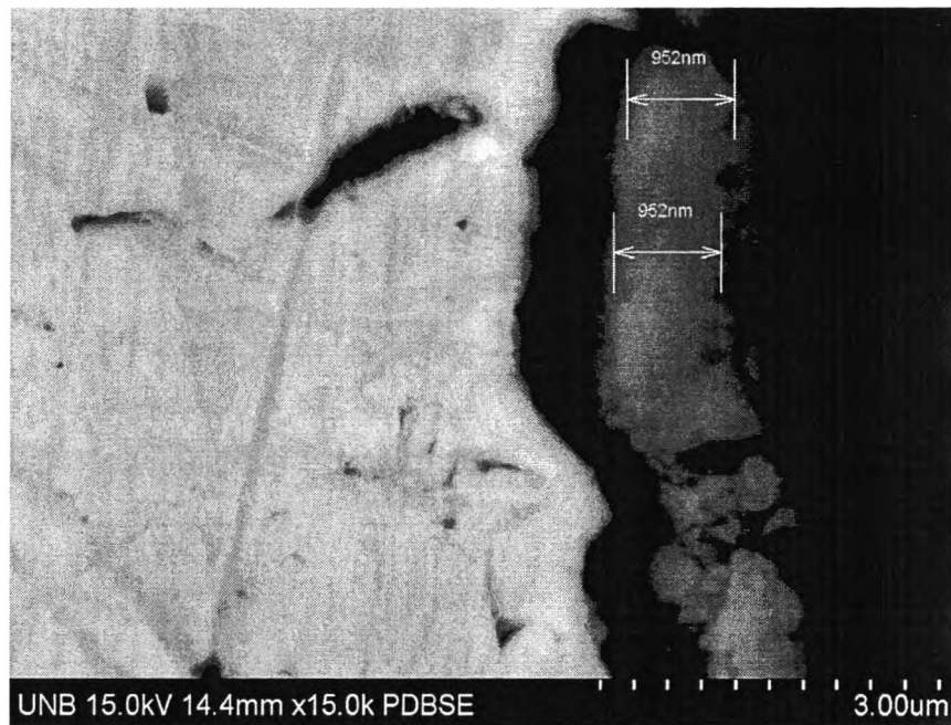
Figure 4.16 Cross-sectional image of the carbon steel membrane (A-side) exposed to 400°C for 1 day.
