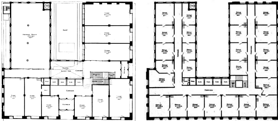
Figure 1: Plans of First and Sixth Floors, Wainwright Building, St. Louis, retrieve from Kindergarten Chats and Other Writings , (Page. 204).
