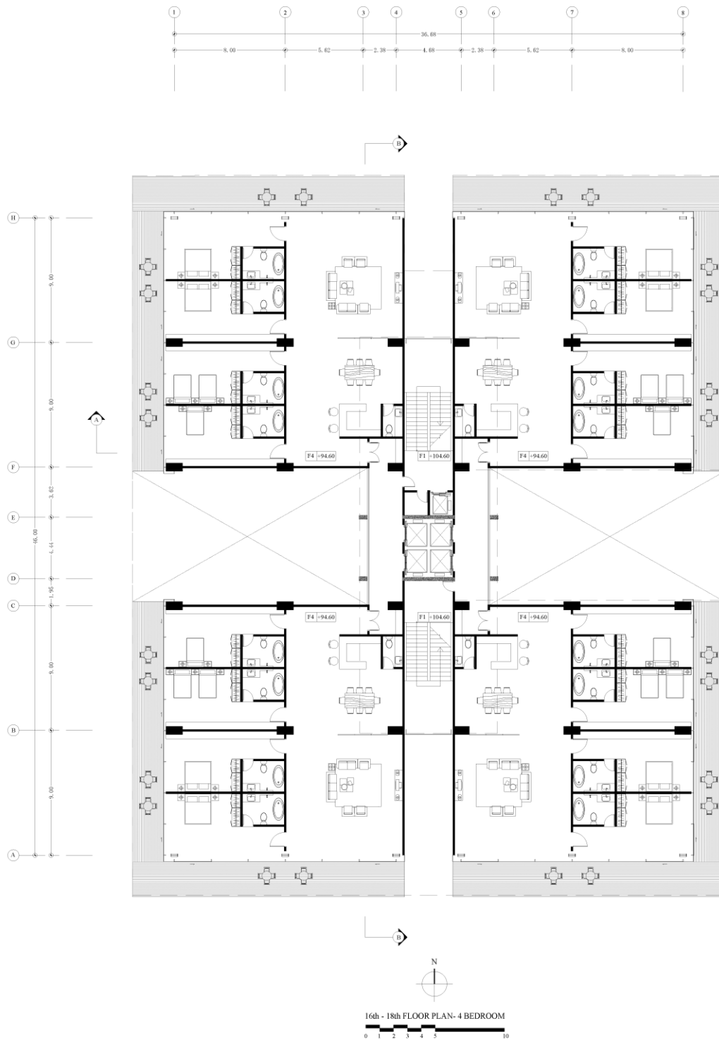
Figure 38: 16 th to 18 th Floor Plan: Four Bedroom Unit, drawn by the author.
