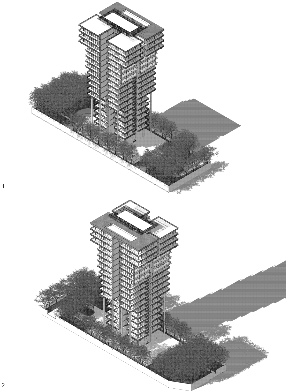
Figure 72: Light and shadow diagram from top to below, Summer Solstice (21 st June) 1. North-East 10:00 AM 2. South-West 5:00 PM, Isometric Views, drawn by the author.
