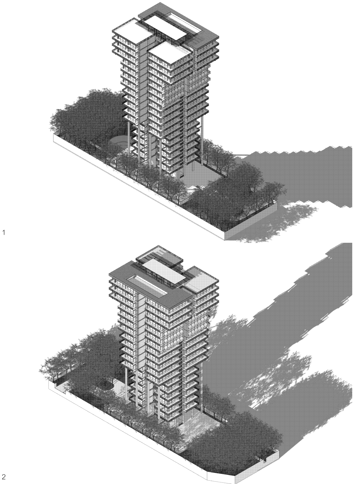
Figure 74: Light and shadow diagram from top to below, Spring Equinox (21 st March)
