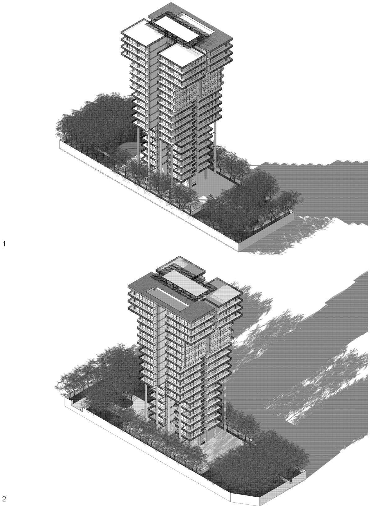
Figure 75: Light and shadow diagram from top to below, Fall Equinox (21 st September)
