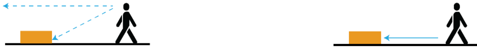
Fig 7: Diagram showing visibility in human eye level, if the plan is cut above that eye level it would overlook the obstacle and generate visibility analysis (Left); And, (Right) diagram showing accessibility, if the plan is cut below the human eye level, it would not overlook the obstacle and generate accessibility analysis.
