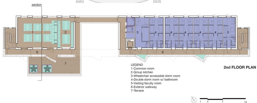
Fig 40: Qualitative typical floor or common space analysis of the ihouse dormitory
