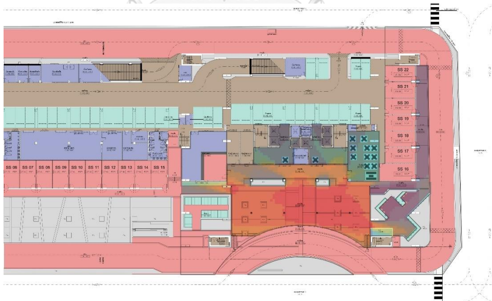
Fig 73: Overlaying qualitative ground floor or the public space with the connectivity analysis from DepthmapX of CU iHouse
