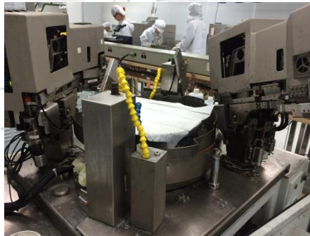
Figure 3.4 Final lapping machine ASL 200
