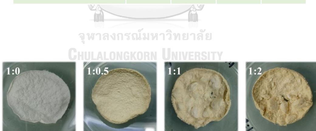
Figure 3.10 QA modified BC prepared from different mole ratio of BC:QA-Cl.
