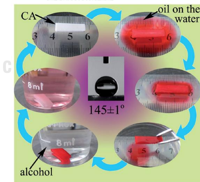
Figure 1.21 The photos show the oil absorption capability of the hydrophobic CAs. 17 mg hydrophobic CAs were placed on the water surface with 150 mL vegetable oil
