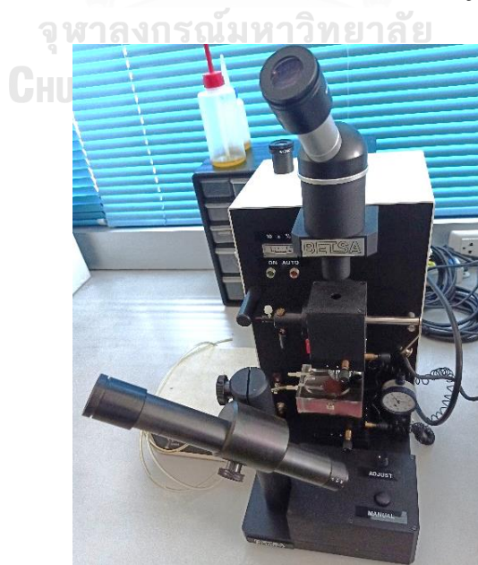
Figure 81: An electric discharge machine (EDM) for drilling the gasket.
