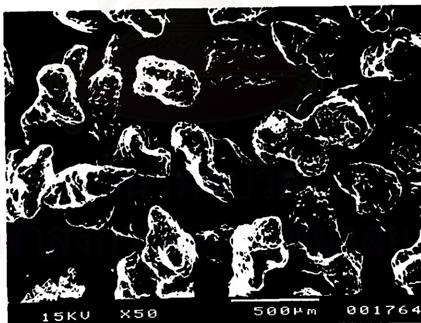
(h) Formulation 9: a core to wall ratio of 1:1, 30% Dibutyl sebacate.
