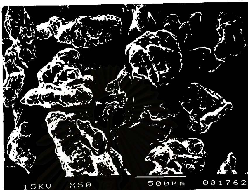
(g) Formulation 8: a core to wall ratio of 1:1, 20% Dibutyl sebacate.
