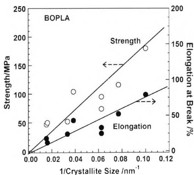
**Figure 4.13** Relationship between the mechanical properties and the inversed crystallite size ((200/110) diffraction) plotted for a series of BOPLA films.
