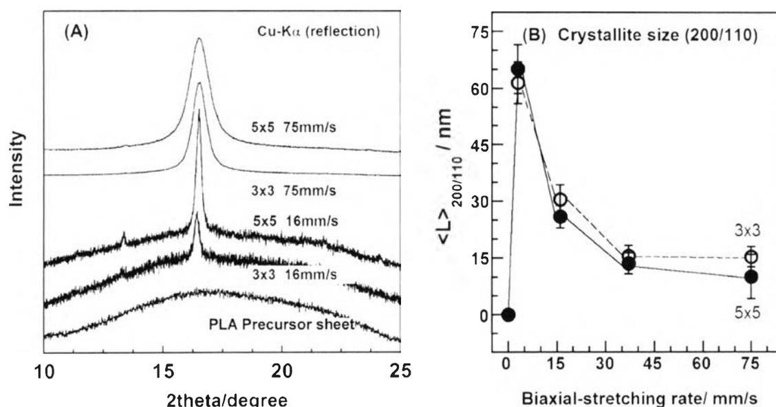
**Figure 4.4** (A) WAXD patterns at room temperature (25 °C) and (B) crystallite size  $\langle L \rangle_{200/110}$  of 3×3-, and 5×5-BOPLA.
