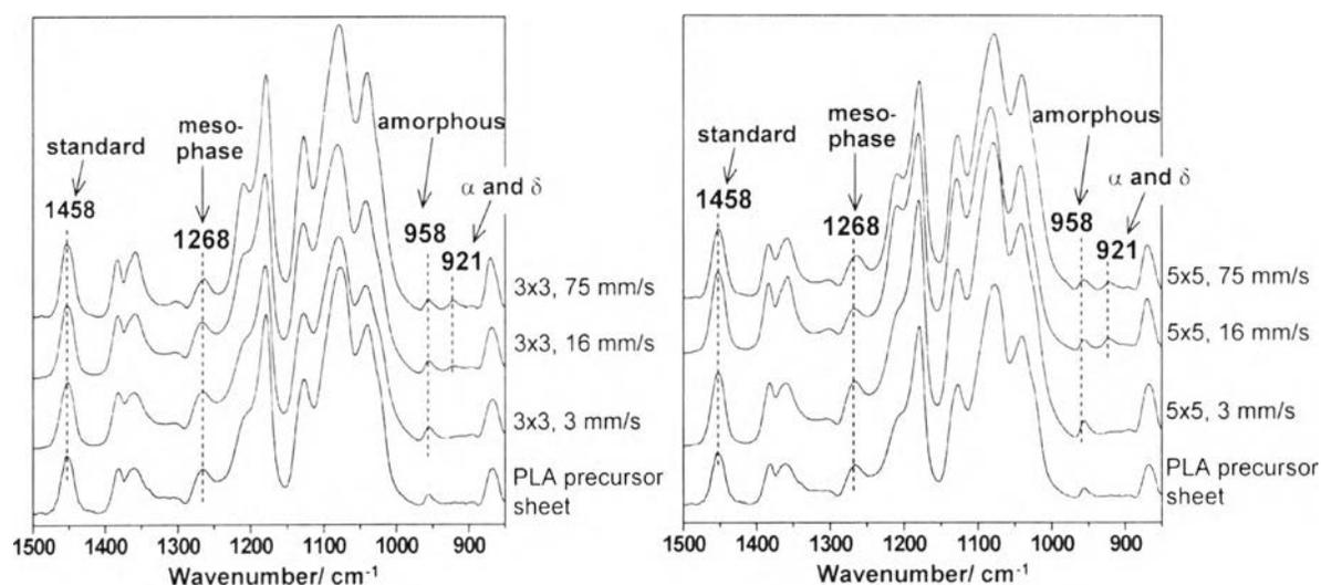
**Figure 4.2** ATR-FTIR spectra of PLA precursor sheet, and 3 $\times$ 3- and 5 $\times$ 5-BOPLA films with varied biaxial-stretching rate.
