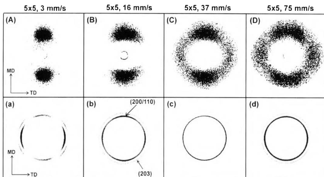
**Figure 4.6** 2D-SAXS (upper) and 2D-WAXD (bottom) patterns of 5×5-BOPLA films produced under various stretching rates.
