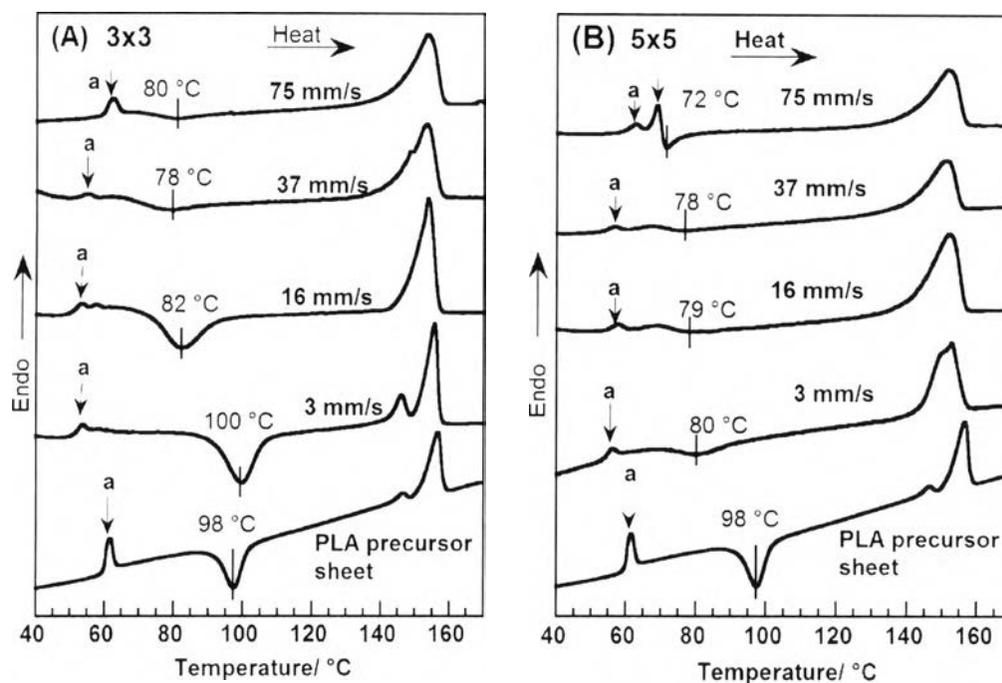
**Figure 4.8** DSC thermograms of BOPLA films at draw ratios of (A) 3×3 and (B) 5×5 by varied stretching rates.
