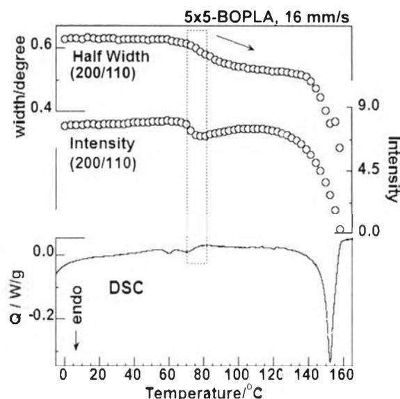
**Figure 4.12** Intensity and half-width of (200/110) diffraction compared with the DSC thermogram measured simultaneously for 5×5-BOPLA at 16 mm/s stretching rate.
