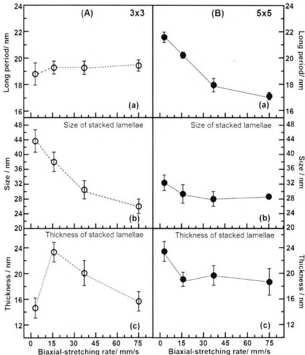
**Figure 4.7** Long period, size and thickness of stacked lamellae as a function of stretching rate for (A) 3×3-, and (B) 5×5-BOPLA films.
