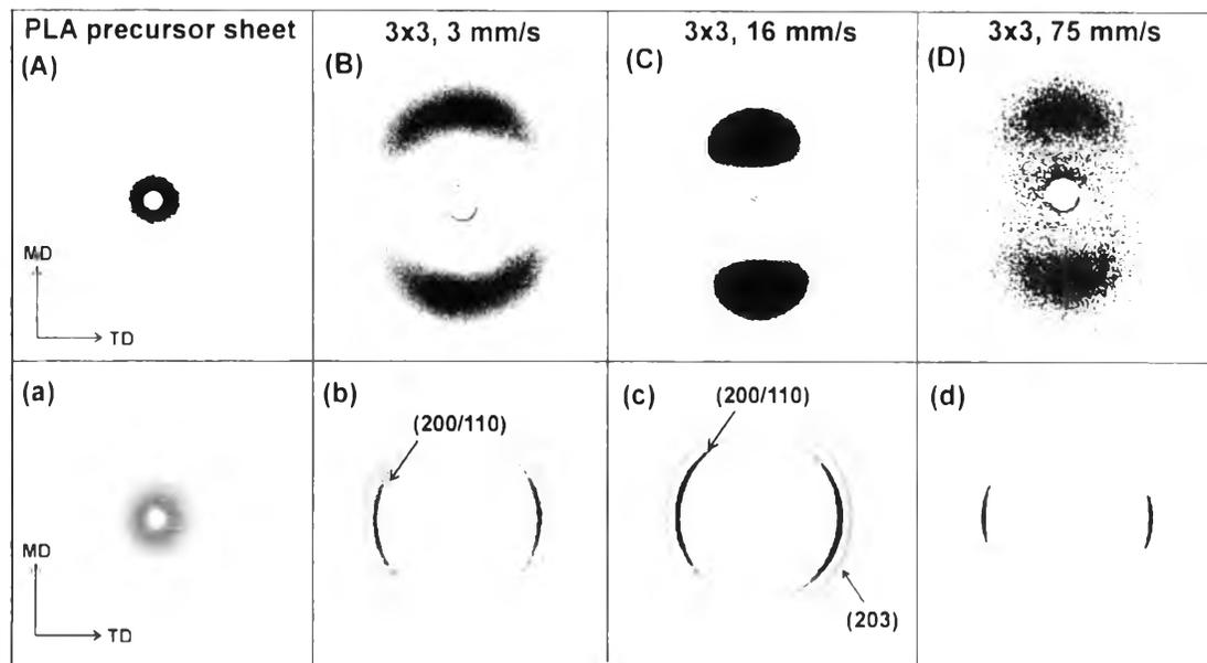
**Figure 4.5** 2D-SAXS (upper) and 2D-WAXD (bottom) patterns of PLA precursor sheet and 3×3-BOPLA films obtained from biaxial-stretching rates of 3, 16, and 75 mm/s, respectively.
