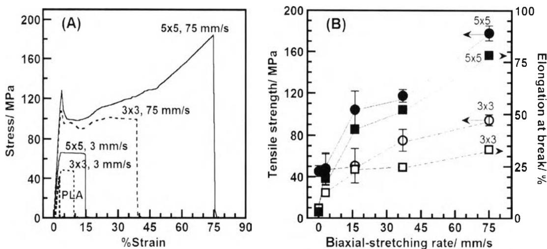
**Figure 4.1** (A) Stress vs strain curves and (B) plots of mechanical properties as a function of biaxial-stretching rate of PLA and BOPLA films.
