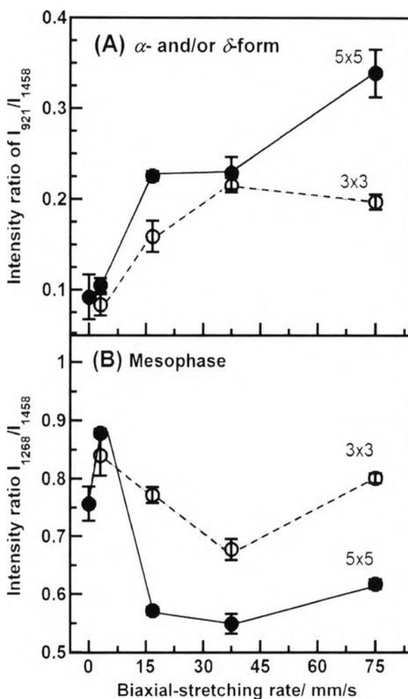
**Figure 4.3** ATR-FTIR peak intensity ratios of crystalline phase and mesophase of various BOPLA films as a function of biaxial-stretching rate.
