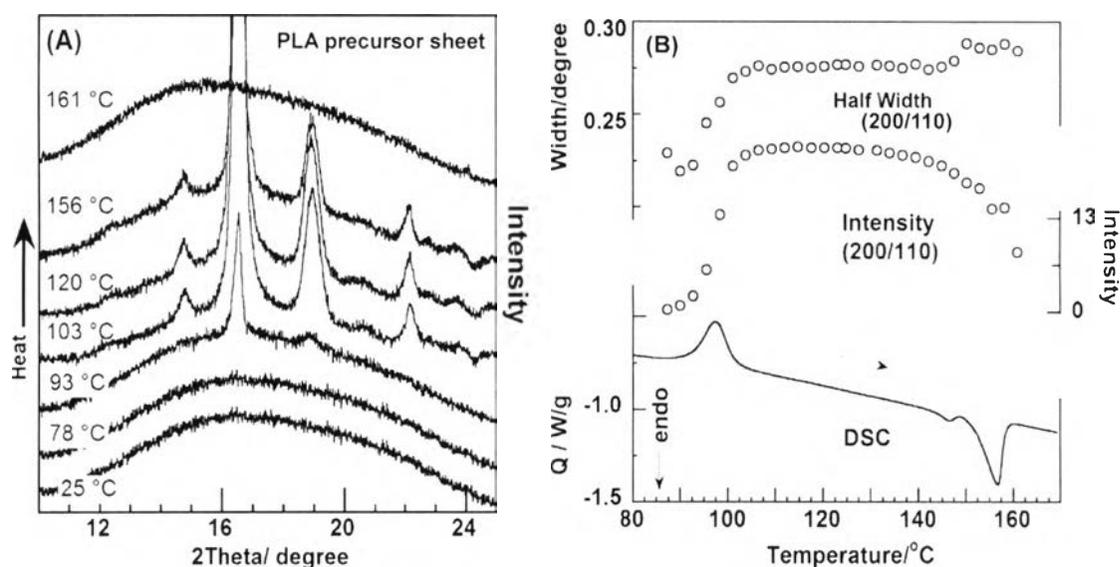
**Figure 4.10** (A) Temperature dependence of WAXD patterns, and (B) DSC thermograms with intensity and half width of (200/110) diffraction for PLA precursor sheet.
