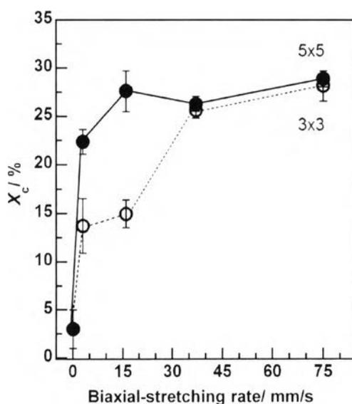
**Figure 4.9** Plots of  $X_c$  derived from DSC thermograms against the stretching rate for 3×3- and 5×5-BOPLA films.
