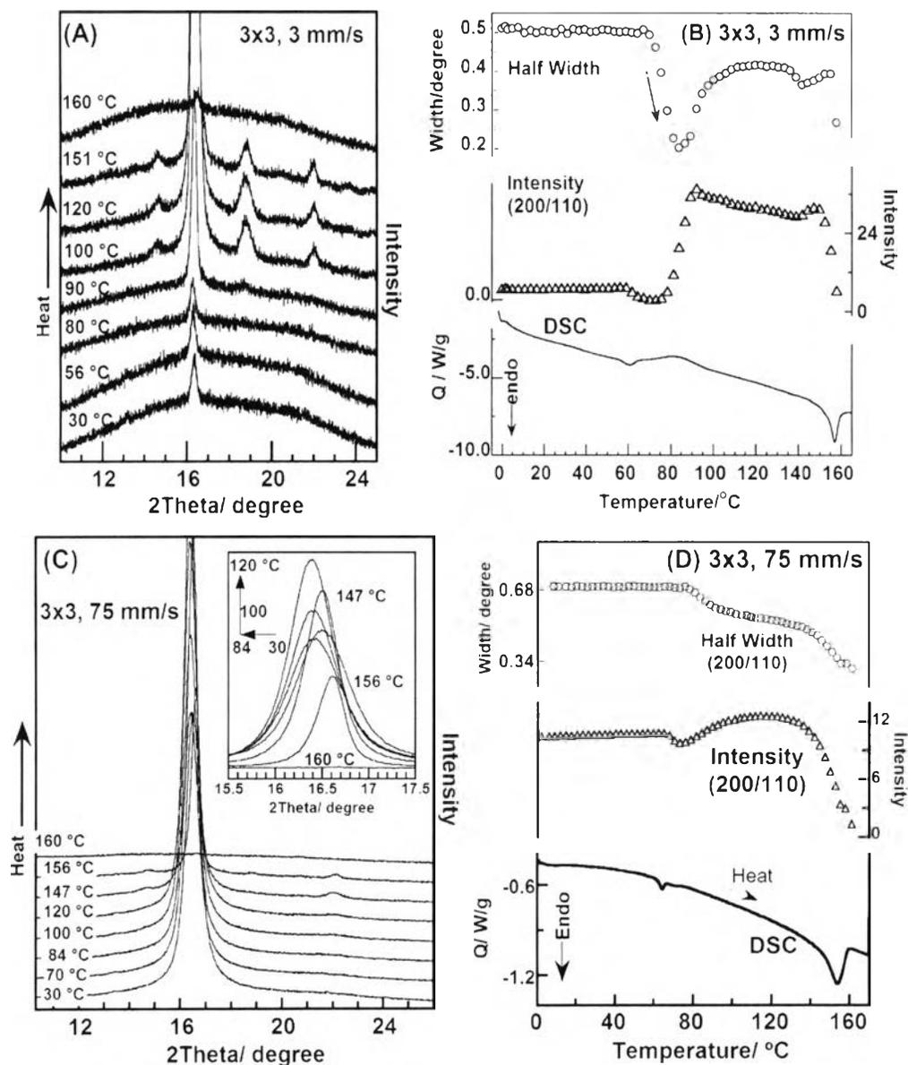
**Figure 4.11** Temperature dependence of WAXD patterns, and intensity and half width of (200/110) diffraction compared with DSC thermograms measured simultaneously for 3x3-BOPLA by (A, B) 3, and (C, D) 75 mm/s, respectively.
