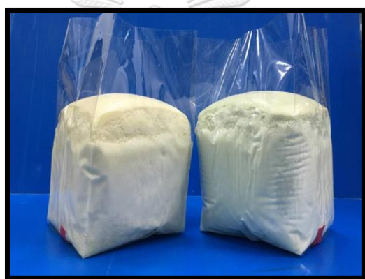
Figure 3.2 RPUR foams prepared by plastic molded method
