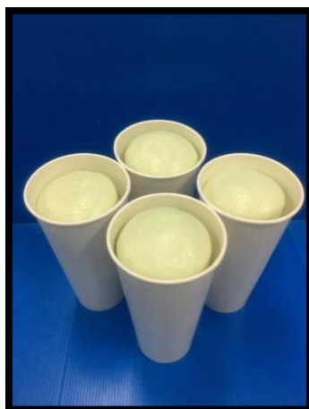
Figure 4.11 RPUR foams prepared by using a 700 ml paper cups
