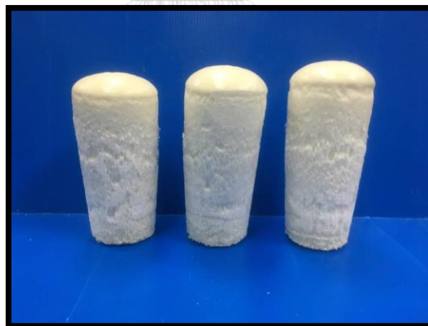
Figure 4.21 Appearance of RPUR foams prepared at different catalyst contents (a) 0.5 pbw, (b) 1.0 pbw and (c) 2.0 pbw
