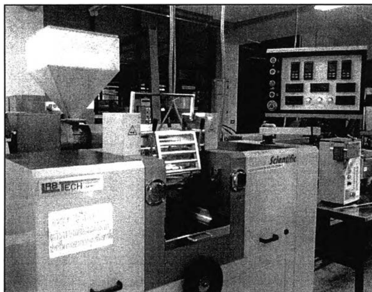
Figure 3.3 Labtech LRM-S-110 Two-roll mill
