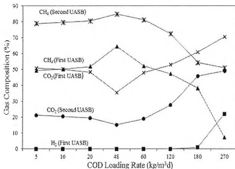
**Figure 4.2** Effect of COD loading rate on gas composition in two-stage UASB.
