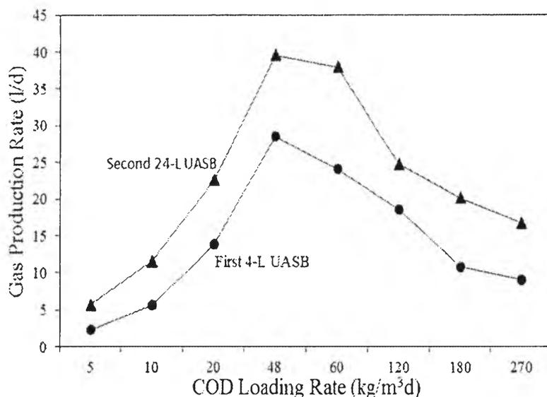
**Figure 4.1** Effect of COD loading rate on gas production rate in two-stage UASB.
