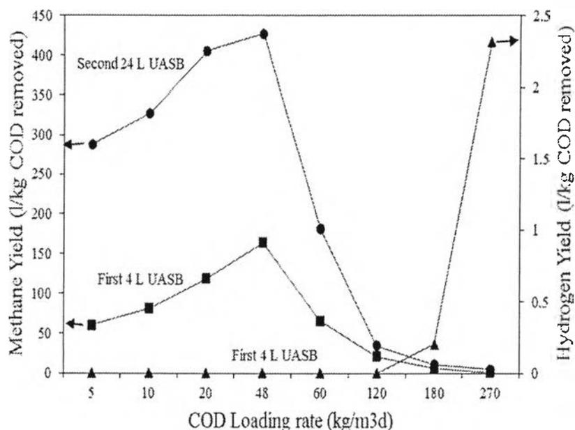
**Figure 4.3** Hydrogen and methane yield versus COD loading rate in two-stage UASB.
