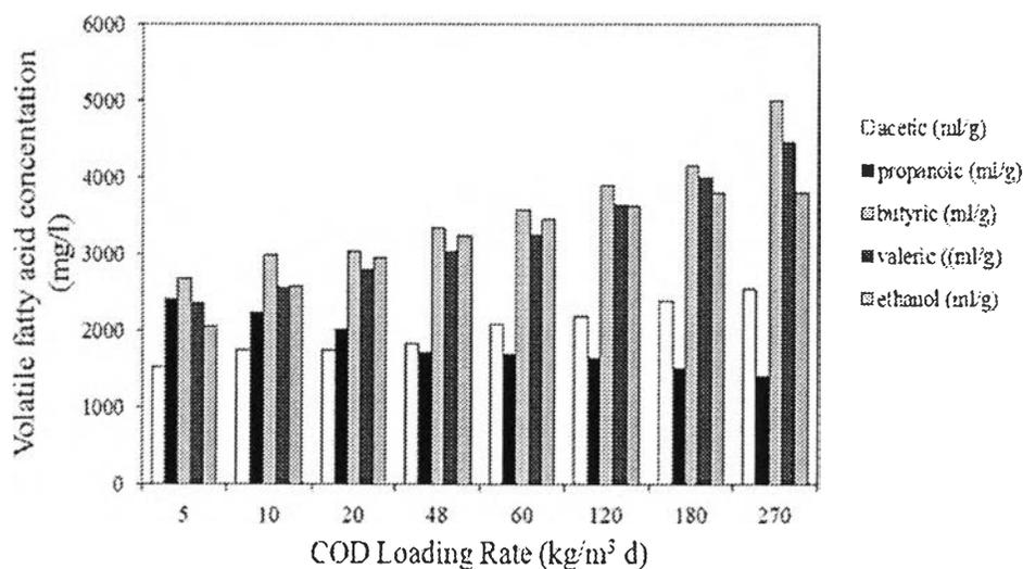
**Figure 4.9** The volatile fatty acid concentration as a function of COD loading rate in a first UASB.
