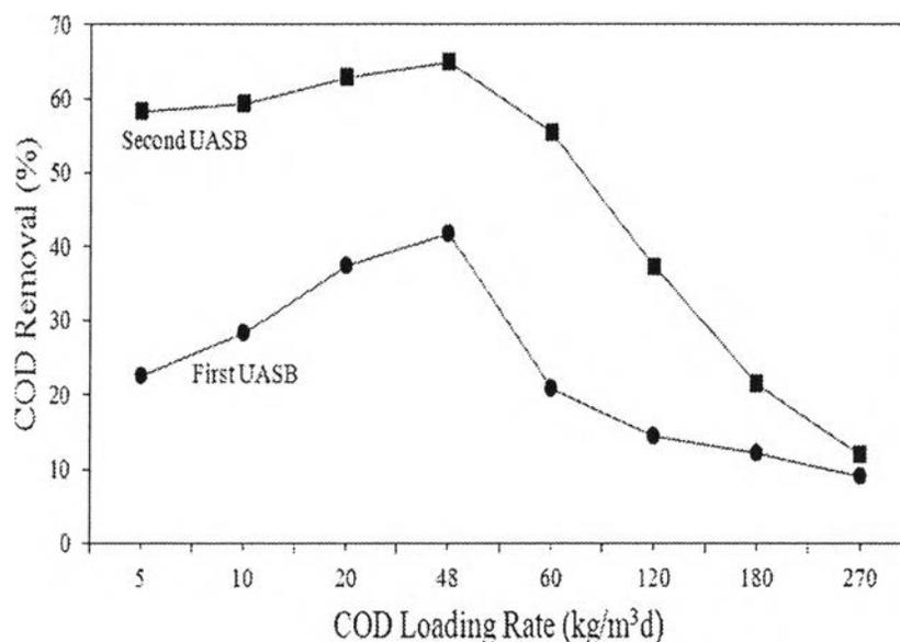
**Figure 4.5** COD removal efficiency versus COD loading rate in two-stage UASB.
