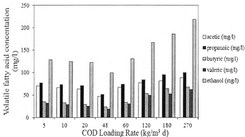
**Figure 4.11** The volatile fatty acid concentration as a function of COD loading rate in a second UASB.
