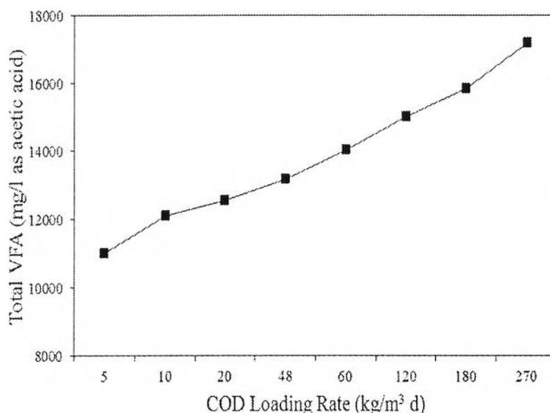
**Figure 4.8** The amount of volatile fatty acid as a function of COD loading rate in a first UASB.
