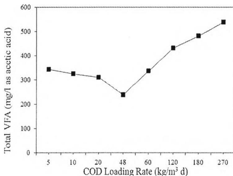
**Figure 4.10** Total volatile fatty acid (VFA) versus COD loading rate in a second UASB.
