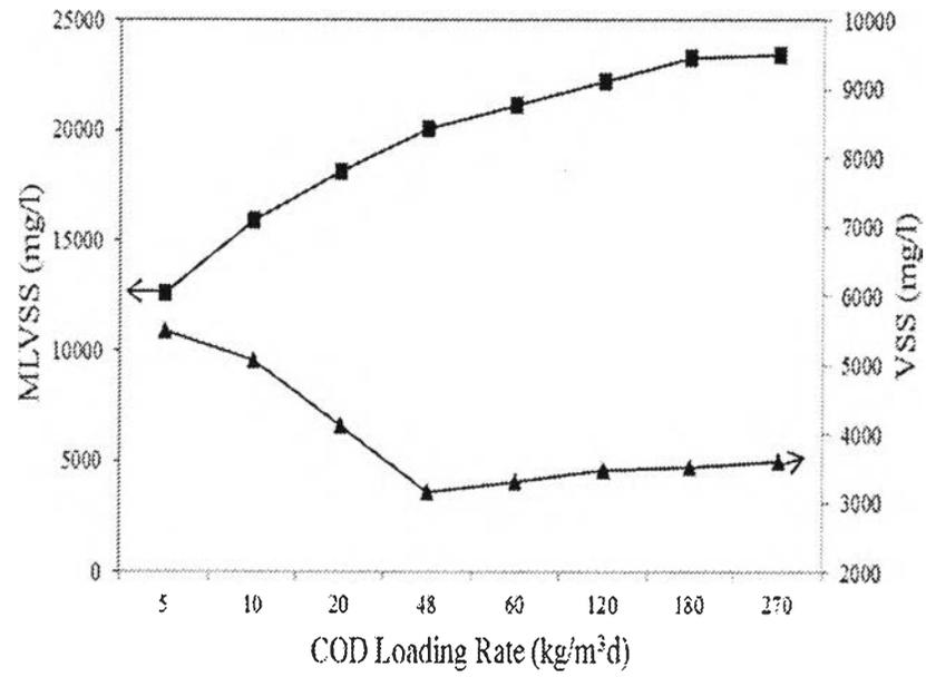
Figure 4.6 MLVSS and effluent VSS versus COD loading rate in a first UASB.
