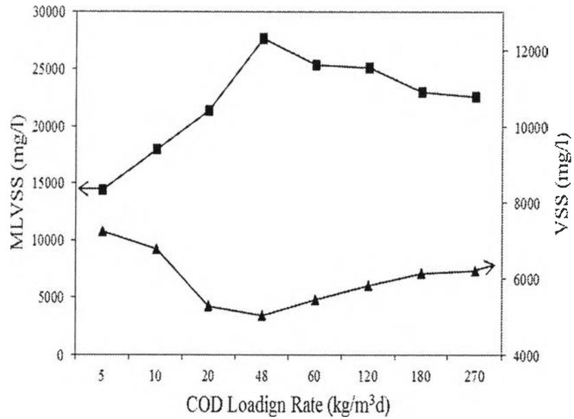
Figure 4.7 MLVSS and effluent VSS versus COD loading rate in a second UASB.
