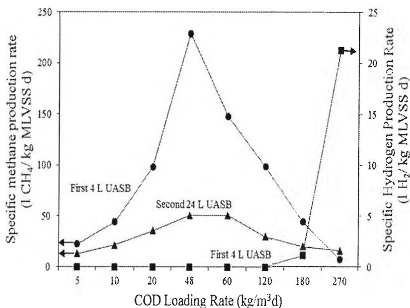
**Figure 4.4** Specific hydrogen and methane production rate versus COD loading rate in two-stage UASB.
