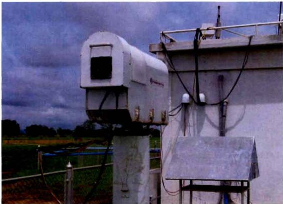
Figure 3.2 The Water vapour Microwave Radiometer WVR 1100 Model (WVR)
