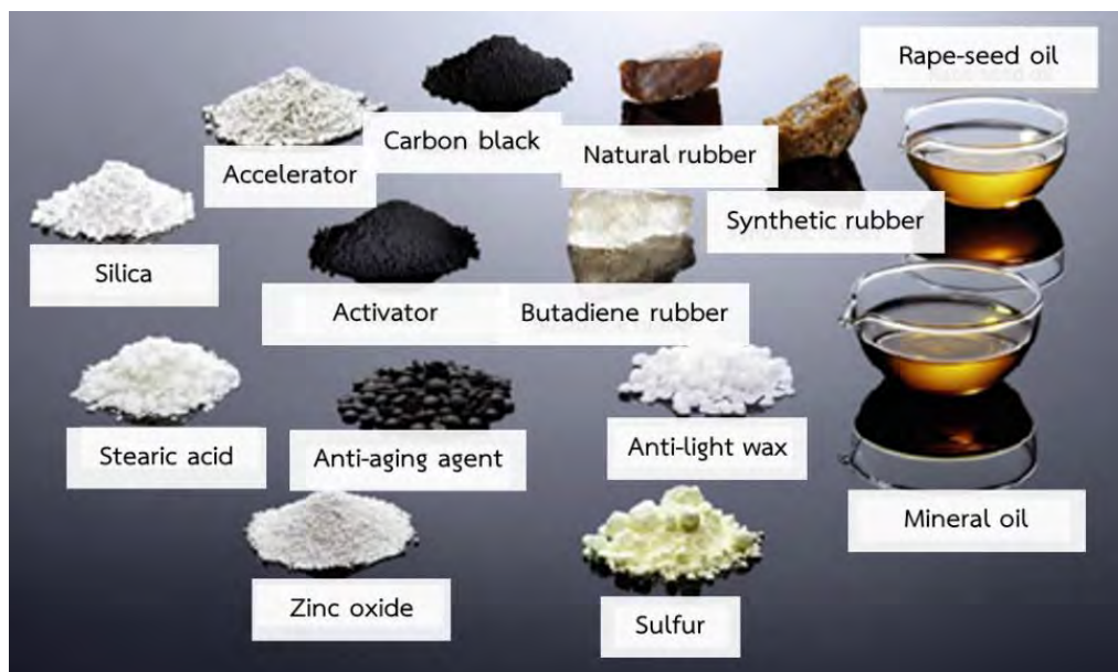
Figure 1.8 The basic components for tire manufacturing [7]
