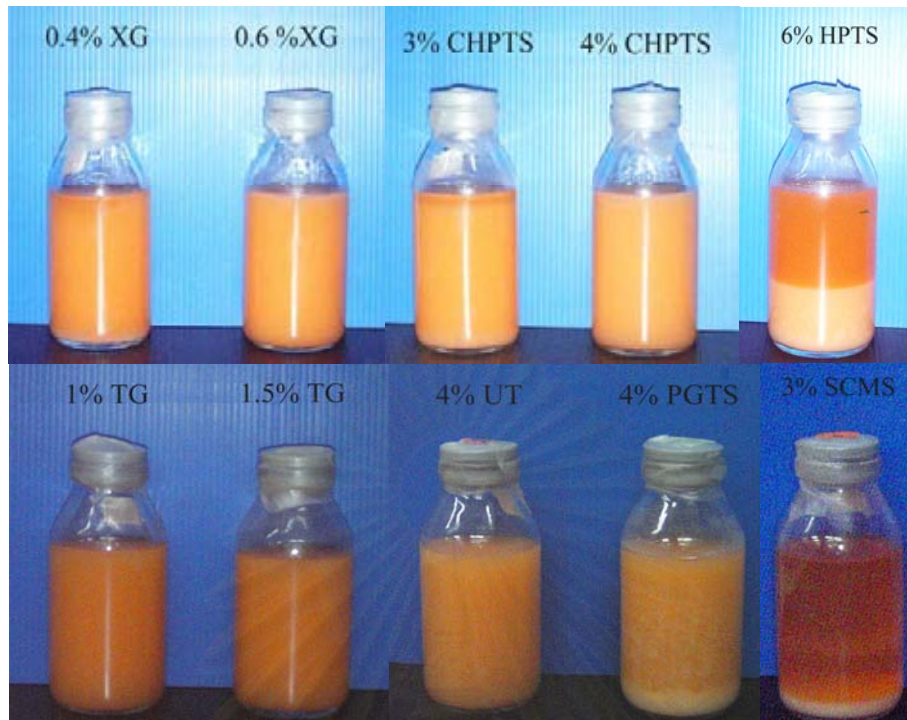
Figure 4-66 Photograph of ibuprofen suspension containing different suspending agents after standing at room temperature for 3 months.
