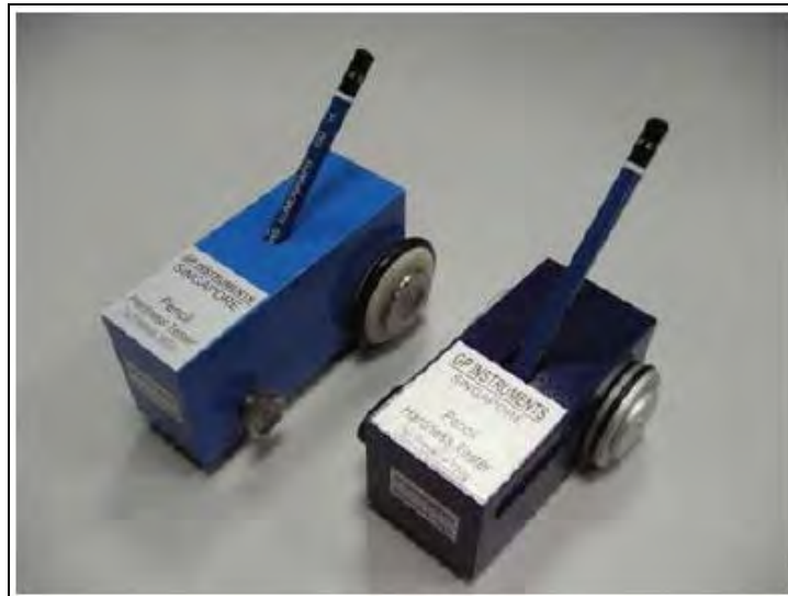
Figure 3.2 Mechanized scratch test apparatus.
