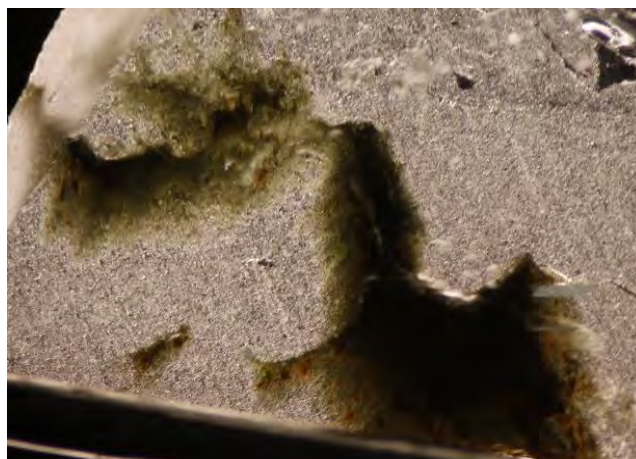
Figure 4.27 Solid inclusions, 1.0X in sample TPNIG002-B from Jos in Nigeria.
