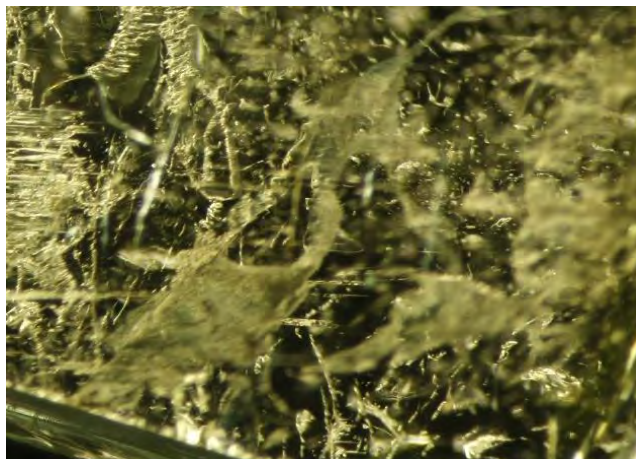
Figure 4.13 Trichites, 1.25X in sample TP MOZ004-A from Nampula in Mozambique.
