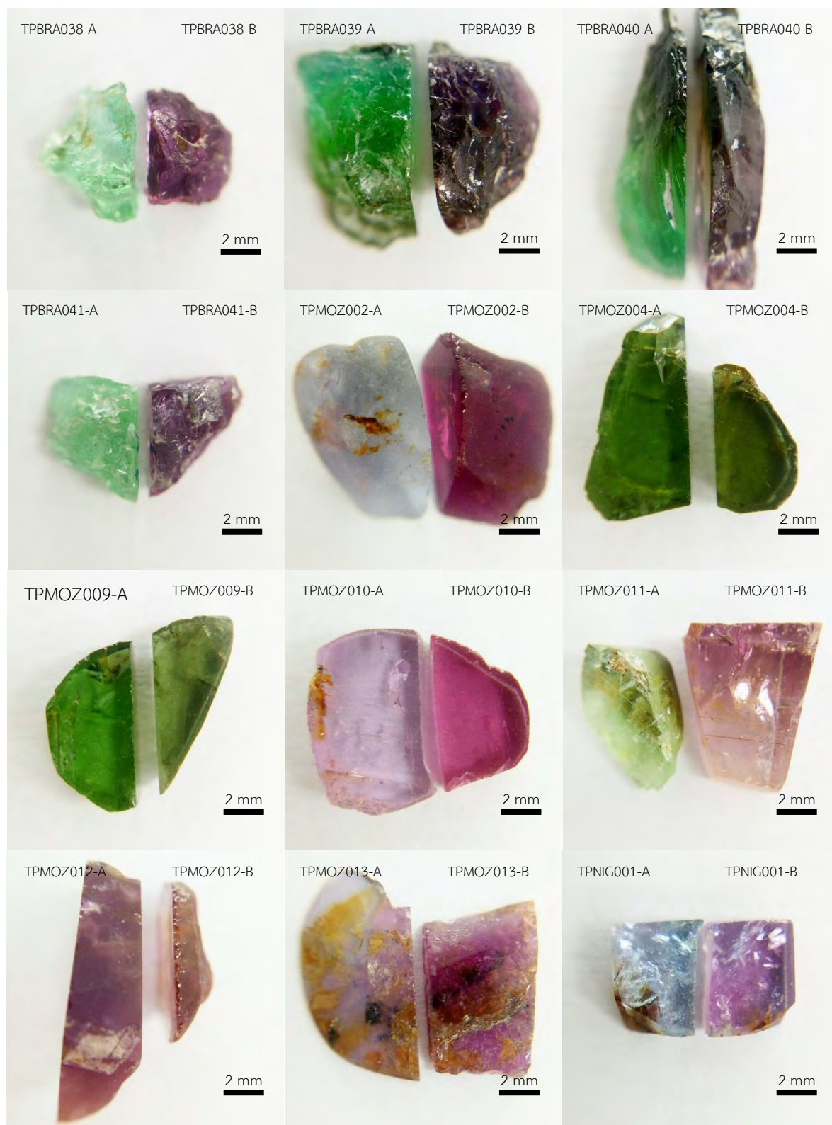
Figure 3.1 Selected twelve tourmalines from Brazil, Mozambique, and Nigeria were cut into 2 pieces which one piece (on the right) of each sample was treated by gamma irradiation (300 kGy) for 2 times.
