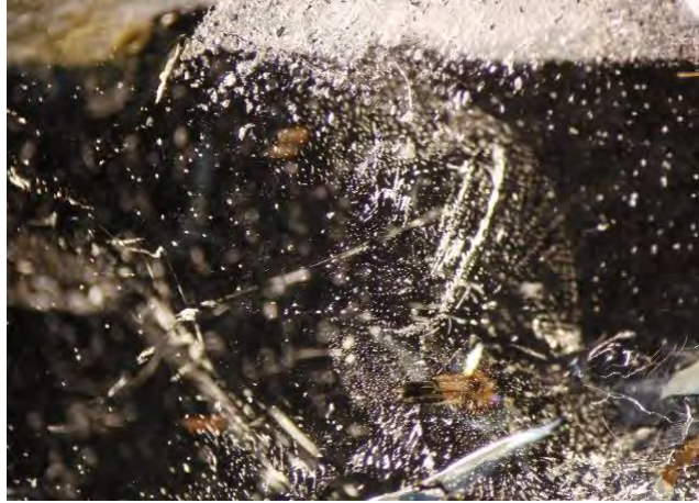
Figure 4.9 Fingerprint inclusions 1.25X in sample TP MOZ007 from Nampula in Mozambique.
