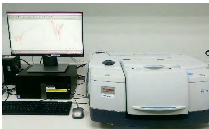
Figure 3.7 Fourier Transform Infrared Spectrophotometer (FTIR) model Nicolet iS50 at ICA GemLab.
