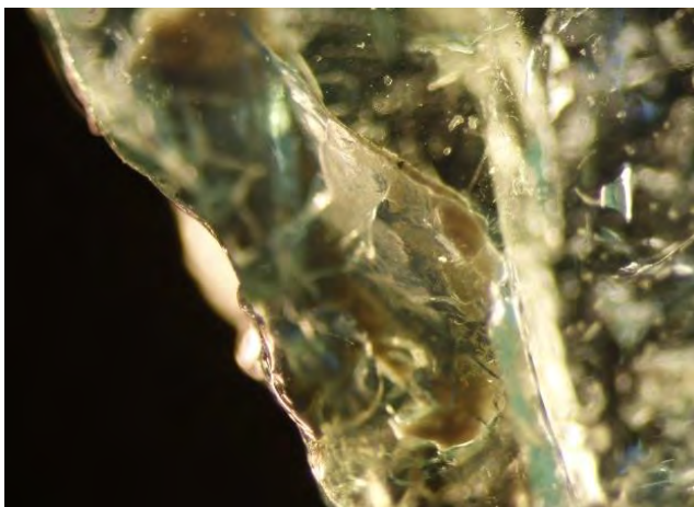
Figure 4.20 Solid inclusions, 2.5X in sample TPBRA037 from Brazil.
