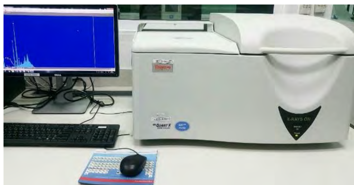
Figure 3.8 Energy-Dispersive X-ray Fluorescence (EDXRF) model ARL QUANT'X at ICA GemLab.
