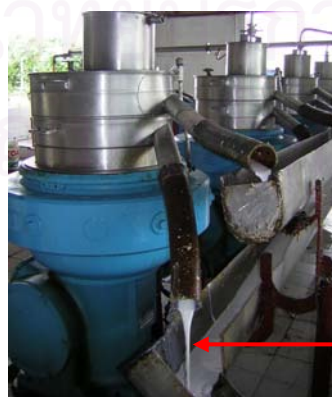
Figure 12. The latex was centrifuged using a factory scale centrifuge at 7,000g to produce the concentrated latex.
