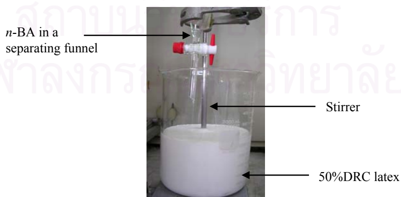
Figure 13 The normal butyl acrylate ( n -BA) was added into 50%DRC latex with slowly continuous stirring.
