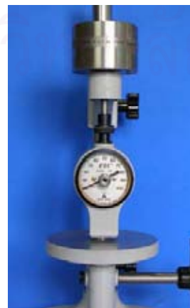
Figure 19. The durometer apparatus was used for measuring the surface hardness.
