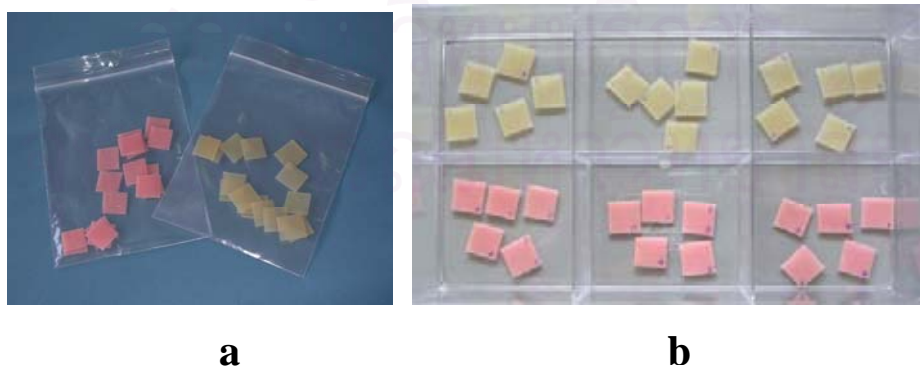
Figure 25 Preparation of the specimens and water absorption test.
