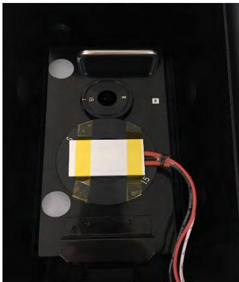
Fig. 3.3.7. Attachment of mini hot plate to the spectrophotometer.
