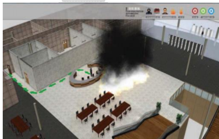
Figure 2.5 BIM-based building evacuation path for evacuation guidance
