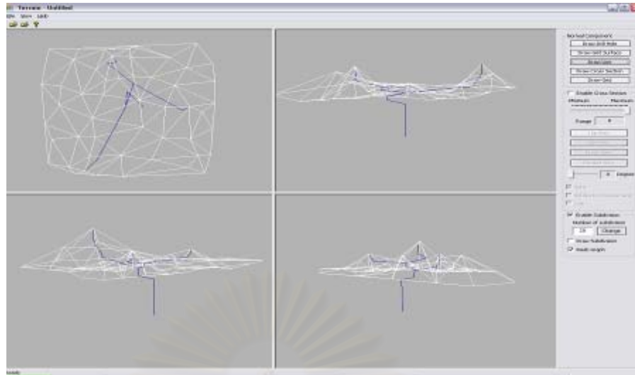
Figure 4.7: Surface reconstruction by creating the Reeb graph
